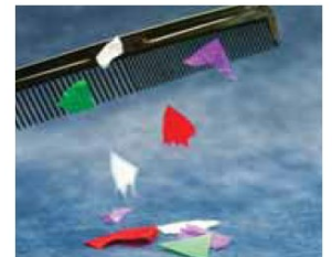
Figure 7.9 Even though the comb is not touching the paper on the table, the paper is attracted to the charged comb.
