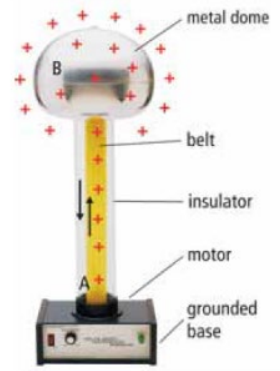
Figure 7.5 Charge is transferred onto a moving belt at the base of the generator, position A, and is transferred off the belt onto the metal dome, position B.
